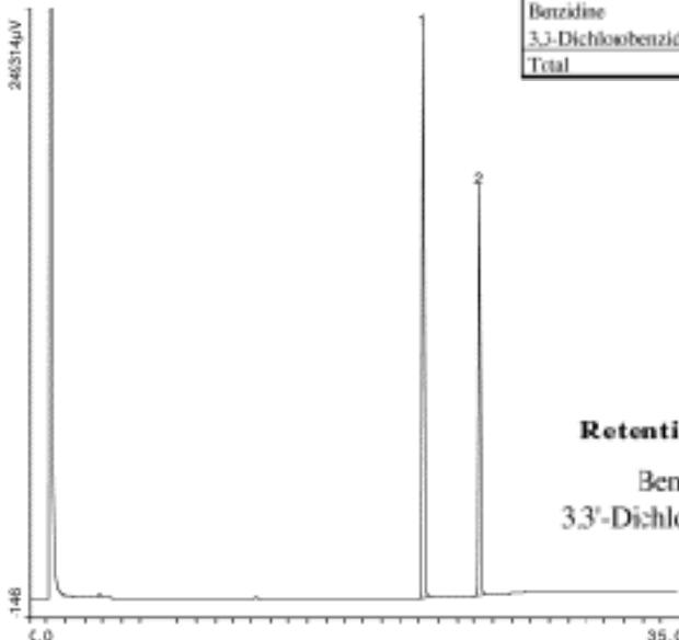
**Method** GC4-M1: Column: SPB-5 (30m X 0.53mm X 1.5 µm film thickness), Flow rates: Helium (carrier) = 10 mL/min., Helium (make-up) = 15 mL/min., Hydrogen (make-up) = 40 mL/min., air (make-up) = 200 mL/min., Temp 1 = 50°C (1 min.), Temp 2 = 300°C (9 min.), Rate = 10°C/min., Injector=200°C, FID=300°C. Analysis performed by Nicole Davis.
