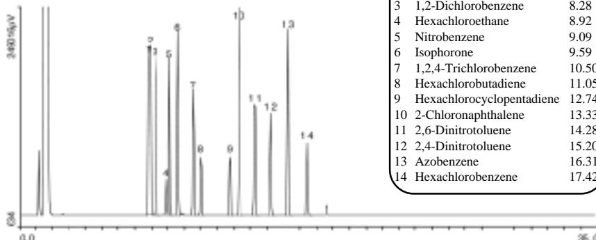
**Method** GC4-M1: Column: SPB-5 (30m X 0.53mm X 1.5  $\mu$ m film thickness), Flow rates: Helium (carrier) = 10 mL/min., Helium (make-up) = 15 mL/min., Hydrogen (make-up) = 40 mL/min., air (make-up) = 200 mL/min., Temp 1 = 50°C (1 min.), Temp 2 = 300°C (9 min.), Rate = 10°C/min., Injector = 200°C, FID = 300°C. Analysis performed by Nicole Davis.
